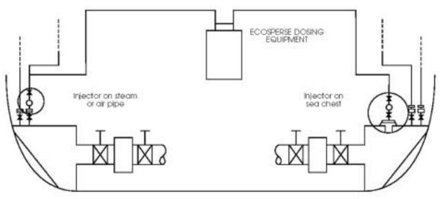
Typical installation of *ECOSPERSE PLUS* dosing equipment Injection point can be fitted also in the sea-chest strainer box
